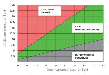
When the ratio between the upstream pressure and the downstream pressure exceeds the 3:1, cavitation of the component occurs. It is then necessary to provide two pressure reducing valves installed one after the other, in order to perform a FIRST LEVEL REDUCTION and then a SECOND LEVEL REDUCTION.
