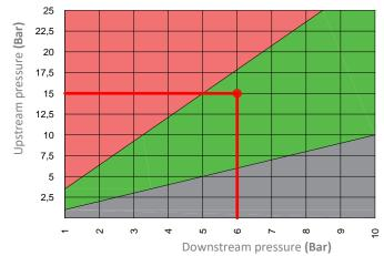
By means of the second reducing valve the pressure will be lowered from 6 bar to 3 bar, with the ideal ratio 6: 3 = 2 (SECOND LEVEL REDUCTION).
